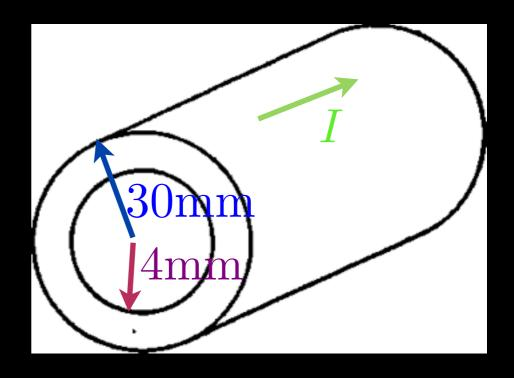
A hollow cylinder with inner radius 4 mm, outer radius 30 mm conducts current I = 3A.
