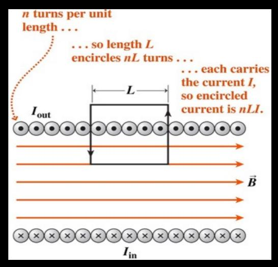
A solenoid used in an MRI scanner is 2.4 m long and 95 cm diameter. It's wound from wire 2.0 mm in diameter. If B = 1.5T, find I.
