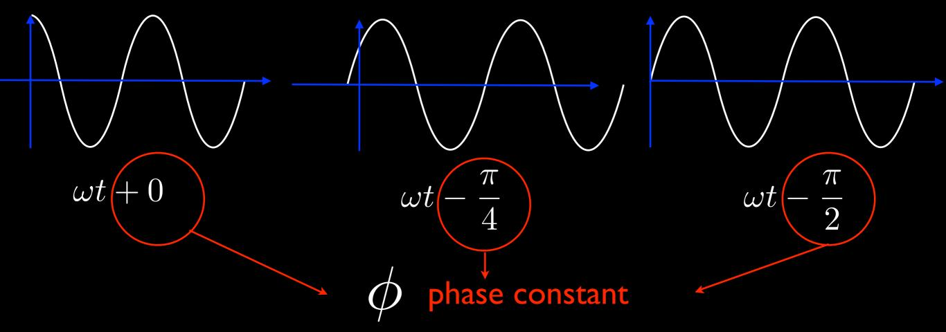
$\phi$  shifts the curve left or right, but does not change A or f.
